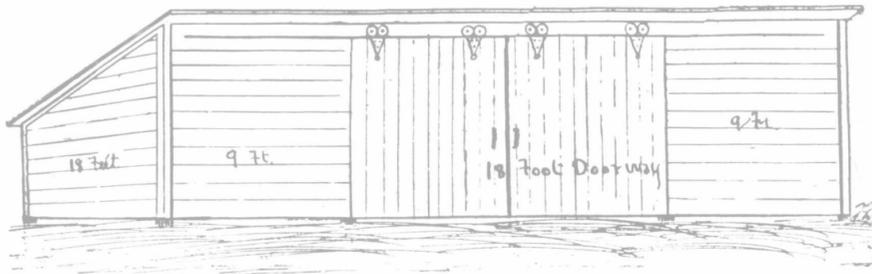
FIG. VI—THIS SHED IS BUILT OF ROUGH LUMBER, NAILED ON POSTS, AND CAN BE PUT UP AT VERY SMALL COST
