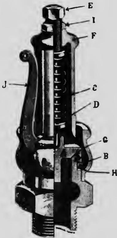
The valve disk A is held to its seat B by the spring C pushing on a spindle D. The pressure on the spring is regulated by the nut E which screws into the case F. The valve disk A has a groove G around its outside rim. As the valve rises it compresses the spring which increases its resistance, and without some provision it would be raised for only a short distance
