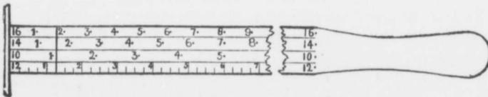
The lower part of the rule is graduated in inches so that the numbers opposite 12 represent inches as well as the number of board feet in boards which are 12 ft. long.
