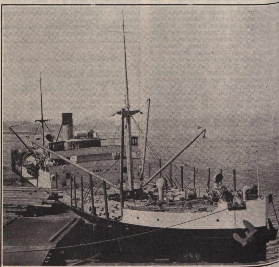
Steel Cargo Steamship, Canadian Exporter, approximately 8,390 d.w. tons, built for Canadian Government Merchant Marine Ltd., by J. Coughlan & Sons, Vancouver, B.C.
