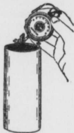
FIG. 40.—B. Testing a dry battery.
