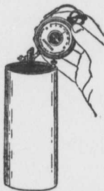
FIG. 40.—B. Testing a dry battery.
