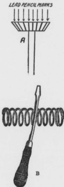
FIG. 72.—A. Testing the seating of a valve. B. Stretching a valve spring.
