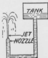
FIG. 34.—A. How the nozzle forms a jet.
