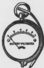
A VOLTMETER FOR TESTING BATTERY CELLS
