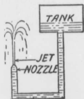
FIG. 34.—A. How the nozzle forms a jet.
