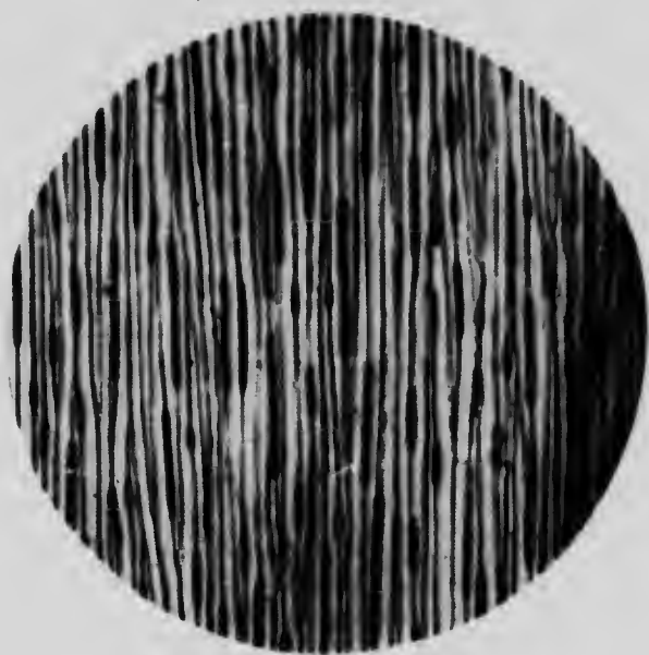
PLATE 43. ABIES NOBILIS . Tangential section showing the character of the medullary rays. \times 46.8
