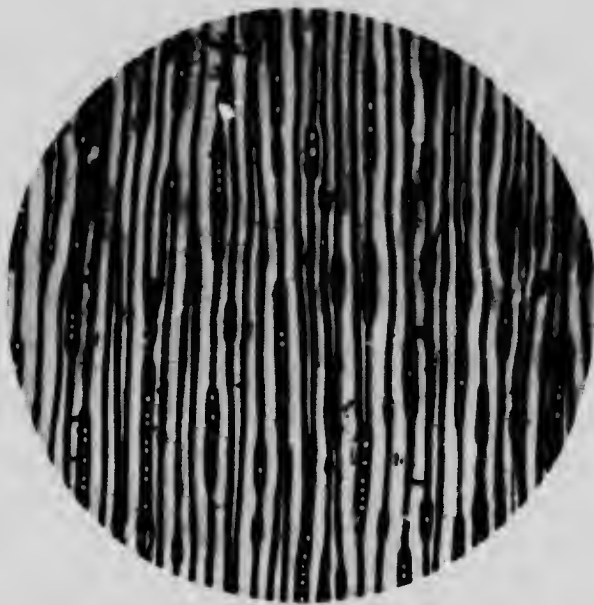
PLATE 33. LIBOCEDRUS DECURRENS . Tangential section showing the character of the rather broad medullary rays and the occurrence of resin. \times 64
