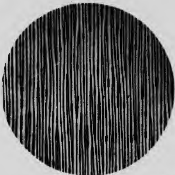
PLATE 35. THUYA OCCIDENTALIS . Tangential section showing the very narrow medullary rays with narrowly oblong cells, taken from the spring wood. \times 64
