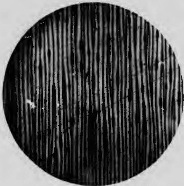
PLATE 27. CRYPTOMERIA JAPONICA . Tangential section showing the character of the low rays in the spring wood. \times 52
