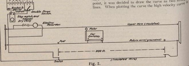
When the meter is suspended from rods, it is, as mentioned before, placed about two feet below the water surface. The rods are firmly held in the arms projecting from the car and very light waterproof electric cable is fastened to the meter for the electric recording circuit. A stay line is also fastened to the meter, when the rods used are light enough to bend when the high velocity runs are being made.
