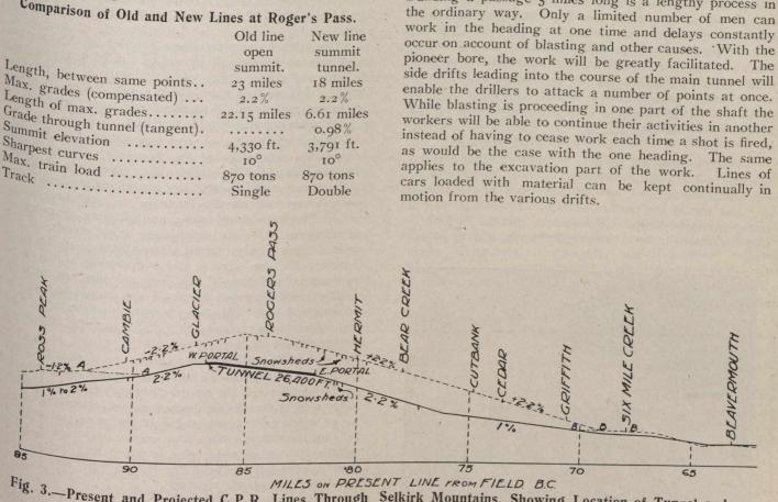
Fig. 3.—Present and Projected C.P.R. Lines Through Selkirk Mountains, Showing Location of Tunnel and Comparison of Grades.
