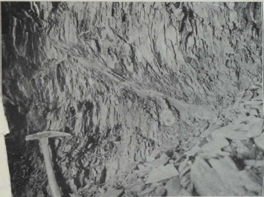
Thrust Fault, showing Phenomenon of Drag in Schist. Looking East, 400 ft. Level, Pearl Lake Mine.
