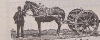
71—R. H.'s Improved Steel Tank Cart. 200 Gallons capacity
