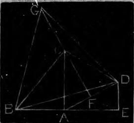
C, draw C F at  $i \le to$  A D, bisecting A D in F. Join E F; join also D B, and on D B describe an equilateral triangle D B G. Then DBG is the triangle required.
