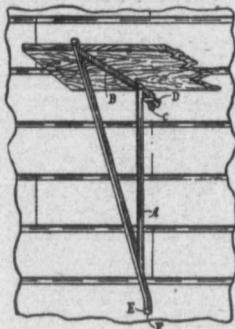
Small Grapppler as used between Vertical Joints of Brickwork.
