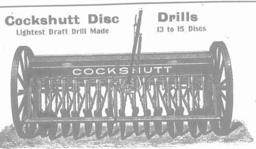
THE great feature of this Cockshutt Disc Drill is its very light draft and even seeding at even depth. The light draft is obtained from self-oiling dust-proof disc bearings and perfect fitting parts. The even seeding is maintained by a protected feed device, not subject to jarring from the wheel action. Seeding at even depth is attained by a steel I-beam frame, which holds up both the discs and grain-box, no matter how rough the usage or wear given the drill.
