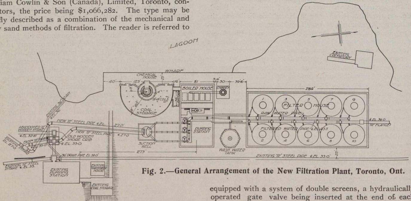
Fig. 2.—General Arrangement of the New Filtration Plant, Toronto, Ont.
