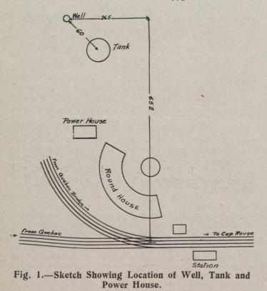
struck in considerable quantity. The hole was then reamed to a diameter of 8-in., and a subsequent test yielded 3,200 imp. gal. per hour.
