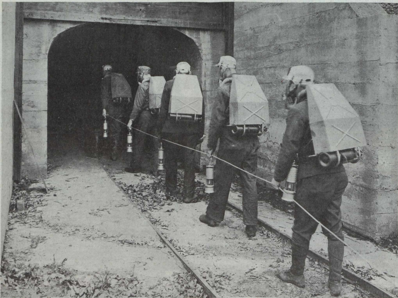
View of the New Oxygen Breathing Apparatus for Mine Rescue Work perfected by the United States Bureau of Mines.
