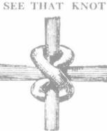
SEE THAT KNOT Made from all No. 9 wire. The STAY WIRE, the LINE WIRE, and the KNOT WIRE.
