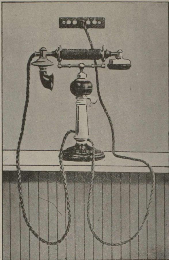
FIG. 3.—ALTERNATIVE TABLE TELEPHONE FOR EXCHANGES
