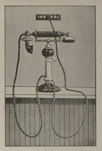
FIG. 3.—ALTERNATIVE TABLE TELEPHONE FOR EXCHANGES IN CENTRAL LONDON.
