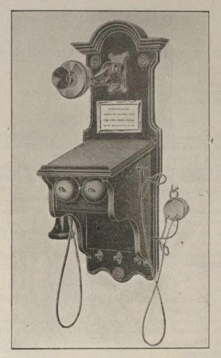
FIG 1.—WALL TELEPHONE FOR EXCHANGES IN CENTRAL LONDON (with moveable arm for adjusting the height of the transmitter).
