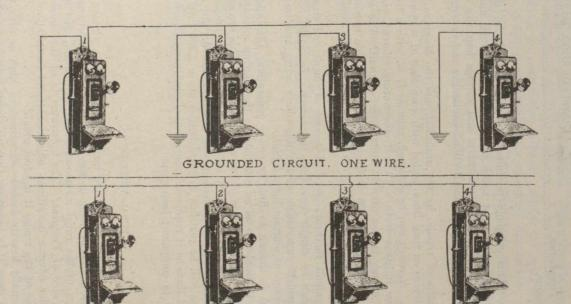
METALLIC CIRCUIT, TWO WIRES.
