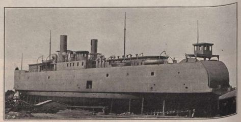
Canadian Northern Railway Car Ferry Steamship Canora, on the ways, showing rolling gate at stern to close in space between decks.
