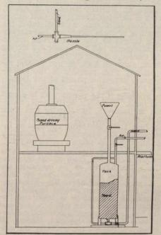
dome casings, driving wheels, or other parts of locomotives, removing all substances right down to bare iron, and thereby giving the opportunity to do the best painting possible.
