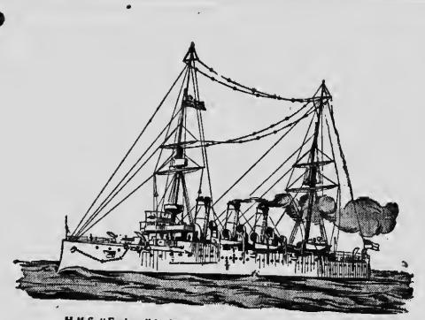
H.M.S. "Furious" in her wireless telegraph and telephone rig. The little stars on these wires represent great wheels of delicate wire, 3 feet in diameter, that catch the electric air-waves.
