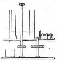
The cylinder through the bottom must be large enough to allow the small wheel by which the machine is driven to pass freely through it, and the tub must be of sufficient diameter to allow of the basket and spindle of the turbine to be freely lifted in and out of it, so that when a charge is done, the basket and spindle may be lifted out, and the sugar emptied out of it, and be replaced ready ion another charge, without jamming in the cylinder and against the sides of the tub.
