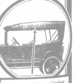
Perfect fitting, "one-man" mohair top; quick adjustable storm curtains, rolled up inside of top.
