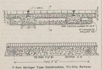
Another advantage of the stone ballast construction is the fact that car service can be turned upon it immediately, whereas any concrete foundation requires about seven days for setting before it can be opened to service.
