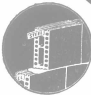
Natco Silo Wall. Note perforated shell, providing firm anchorage for mortar joints.
