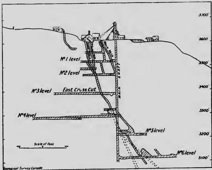
Figure 26. Transverse (east and west) projection through Velvet mine, Rossland, B.C.
