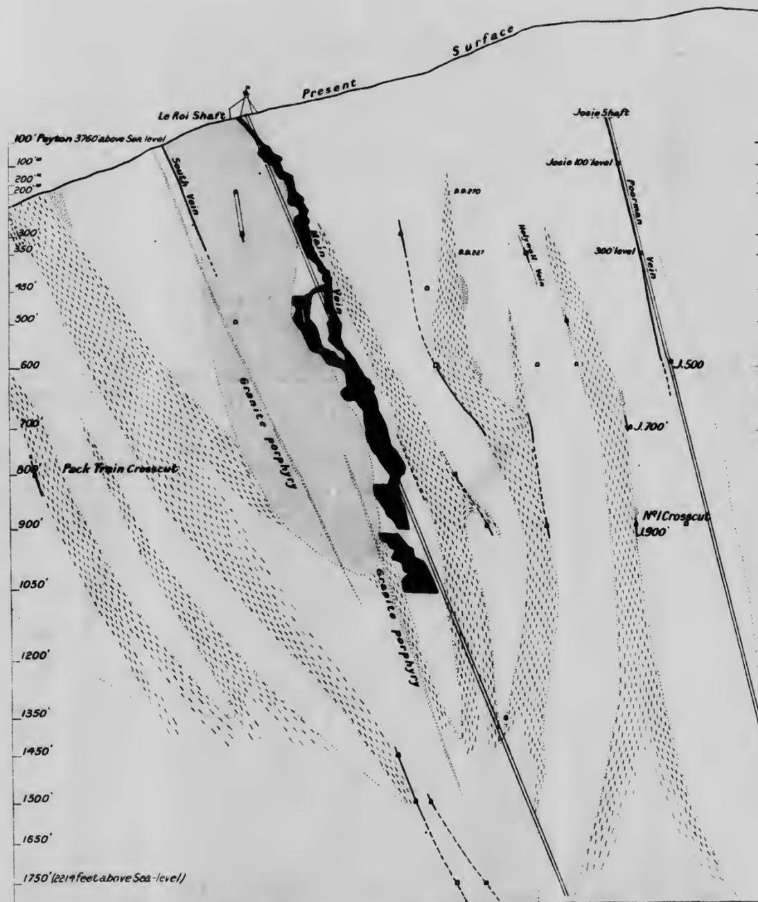
Vertical Section G-D through Le Roi Mine 125 feet east of Main Shaft
