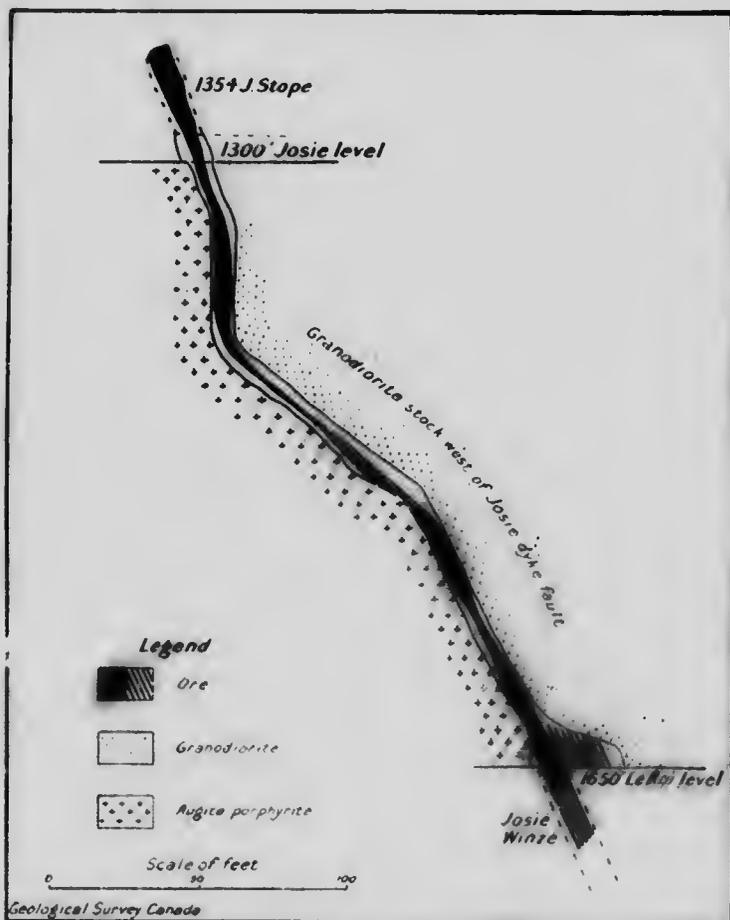
Figure 7. Transverse vertical section through No. 1687 raise, LeRoi mine, Rosland, B.C.
