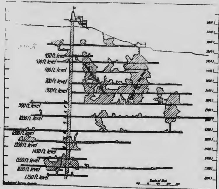
Figure 19. Longitudinal projection of the South vein, LeRoi mine, Rossland, B.C.
