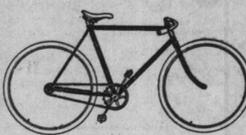
MODEL 7, "HARTFORD," chain wheel, height of frame, 22, 24 and 26-inch, dropped crank bracket, narrow tread, 28-inch wheels, fitted with Hartford single tube tires and "Columbia" New Departure brake, gear 72 to 82, made and guaranteed by the Pope Manufacturing Co. of Hartford, Conn., strictly up to date. \$30.00
