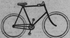
MODEL 57, "COLUMBIA," chain wheel, 22, 24-inch frame, improved flush joint, 2 1/2-inch dropped crank bracket, narrow tread, narrow rear forks, 28-inch wheels, rims enameled black with gold stripes, No. 80 Hartford or Dunlop tires, 3-16-inch chain, 7-inch cranks, combination pedals, reversible steel handle-bars, internal expander, Columbia New Departure brake, gear 72 to 82, weight 27 1/2 lbs. \$55.00
