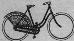
MODEL 58, "COLUMBIA," chain wheel, 20, 22, 24-inch frame, improved flush joint, 2 1/2-inch dropped crank bracket, narrow tread, narrow rear forks, 28-inch wheels, rims enameled black with gold stripes, Hartford single tube tires, or Dunlop external expanders, wood rear wheel and chain guards, Columbia New Departure brake, gear 68 to 72. \$55.00
