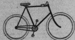
MODEL 57, "COLUMBIA," chain wheel, 22, 24-inch frame, improved flush joint, 2 1/2-inch dropped crank bracket, narrow tread, narrow rear forks, 28-inch wheels, rims enameled black with gold stripes, No. 80 Hartford or Dunlop tires, 3-16-inch chain, 7-inch cranks, combination pedals, reversible steel handle-bars, internal expander, Columbia New Departure brake, gear 72 to 82, weight 27 1/2 lbs. \$55.00
