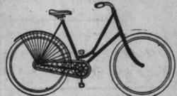
MODEL 8, LADIES "HARTFORD" bicycle, height of frame, 20, 22 and 24-inch, 28-inch wheels, 6 1/2-inch cranks, rubber pedals, New Departure brake, 1 1/2-inch tubing, gear 66 to 72, Hartford single tube tires, handsome in appearance and as durable a wheel as there is manufactured, and fully guaranteed. \$30.00
