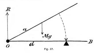
Let the rod (Fig. 37) drop from the vertical position and strike an obstacle when in the position OB with a blow Q. Let R be the impulse on the fixed end O, and then we have, taking moments about O, ir
