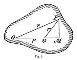
Let the plane of Fig. 5 represent any plane of the body perpendicular to the two parallel axes, of which one cuts this plane in the point O, and the other passing through the centre of inertia cuts it in G. Then for any point P in this plane, we have
