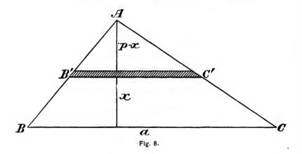
In Fig. 8, divide the triangle into strips of mass  $\rho y dx$ , where y = B'C'.
