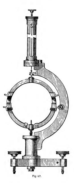
It may be observed also that if the gyroscope be given no initial impulse, but be merely let drop, it will act in the same manner as a top, and oscillate up and down while it keeps in motion about the vertical.
