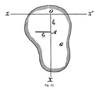
no strain upon the axis about which it is free to rotate? Let the body (Fig. 32) surround O; let ZZ' be the axis of rotation, and let the plane of zx, which is the plane of the paper, contain G, the centre of inertia of the body. Suppose that the blow Q is applied at the point whose coördinates are  $\xi$ ,  $\eta$ ,  $\zeta$  (the coördinate  $\eta$  not being shown, being drawn upwards perpendicular to the plane of the paper). If there be no resulting
