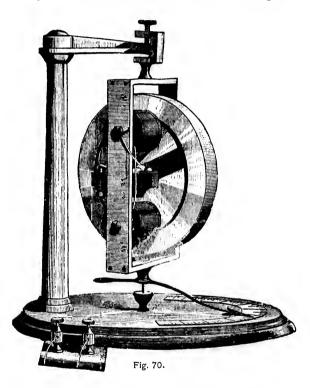
The rectangular frame which contains the wheel is supported by a fine and very hard steel point, which rests upon an agate step in the bottom of a small iron cup at the end of the arr that is supported by the standard. The wheel spindle turns on carefully made steel points, and upon it are placed two cams, one ar each end, which operate the current-breaking springs.
