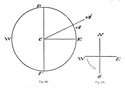
represents the tangent plane at A, to an observer at A' above the gyroscope, the earth will move from west to east as indicated by the arrow, and the apparent motion of the index attached to the gyroscope will be as before from east to west.
