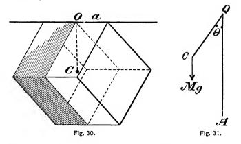
Figs. 30 and 31 show the motion. Since the body and forces are symmetrical about the central plane perpendicular to the axis of rotation, the pressures on the axis, as the cube swings
