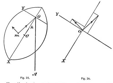
Now, if  $\omega$  be the angular velocity, any particle such as m will be acted on by the forces  $m\omega^2 r$ ,  $m\dot{\omega}r$ , as is indicated in the figure; and these forces resolved along OX, OY, as shown in Fig. 26, would give
