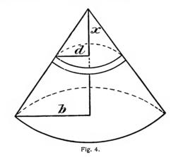
Dividing the cone up into circular strips, perpendicular to its axis, as in Fig. 4, we have, if a be its height,
