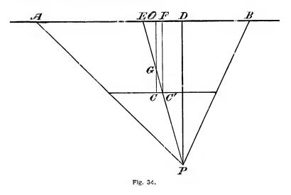
Fig. 34 shows the position of the centre of percussion. AB is the rotation axis, PD perpendicular to AB, E the middle point of AB, F the middle point of DE. Then AB is a principal axis at the point F, and G being the centre of inertia of the plate, and PD=p,
