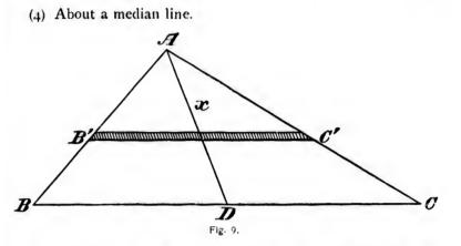
In Fig. 9, divide the triangle into strips parallel to *BC*, as before, and let y = B'C'. Then the mass of a strip is  $\rho y dx \sin D$ , and its moment of inertia about *AD* is  $\rho y dx \sin D \cdot \frac{y^2}{12} \sin^2 D$ .
