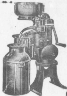
Note the heavy compact construction and convenient height of supply can and discharge spouts. The top of the supply can is only 3½ feet from the floor.
