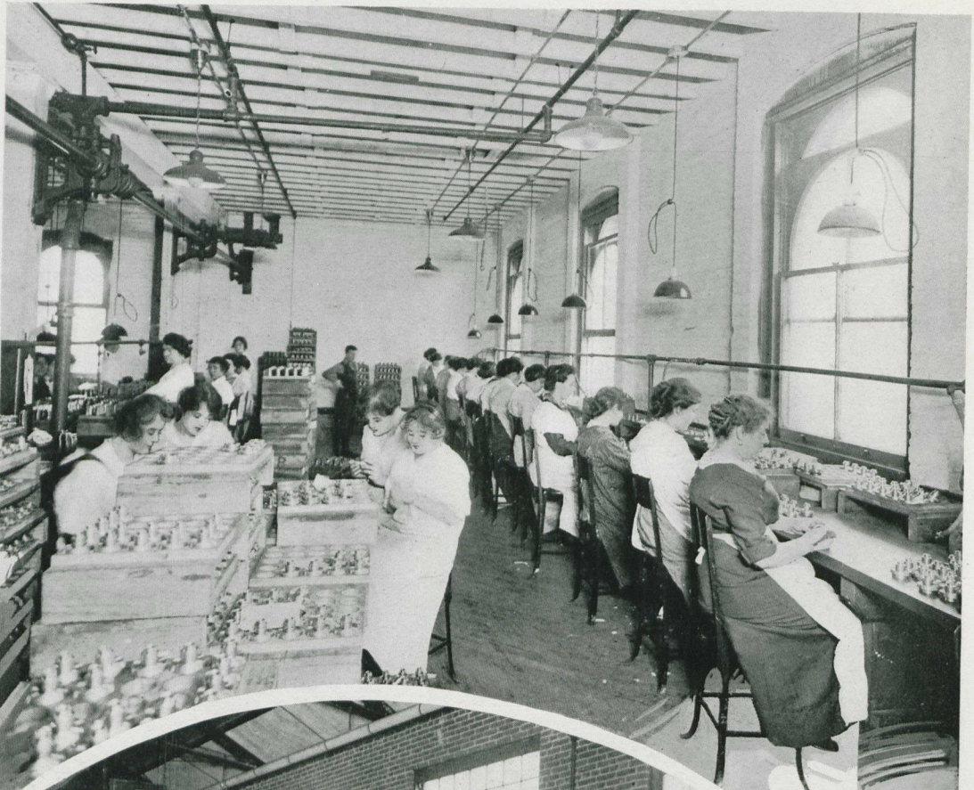
Inspection of Bodies No. 100 Fuse
