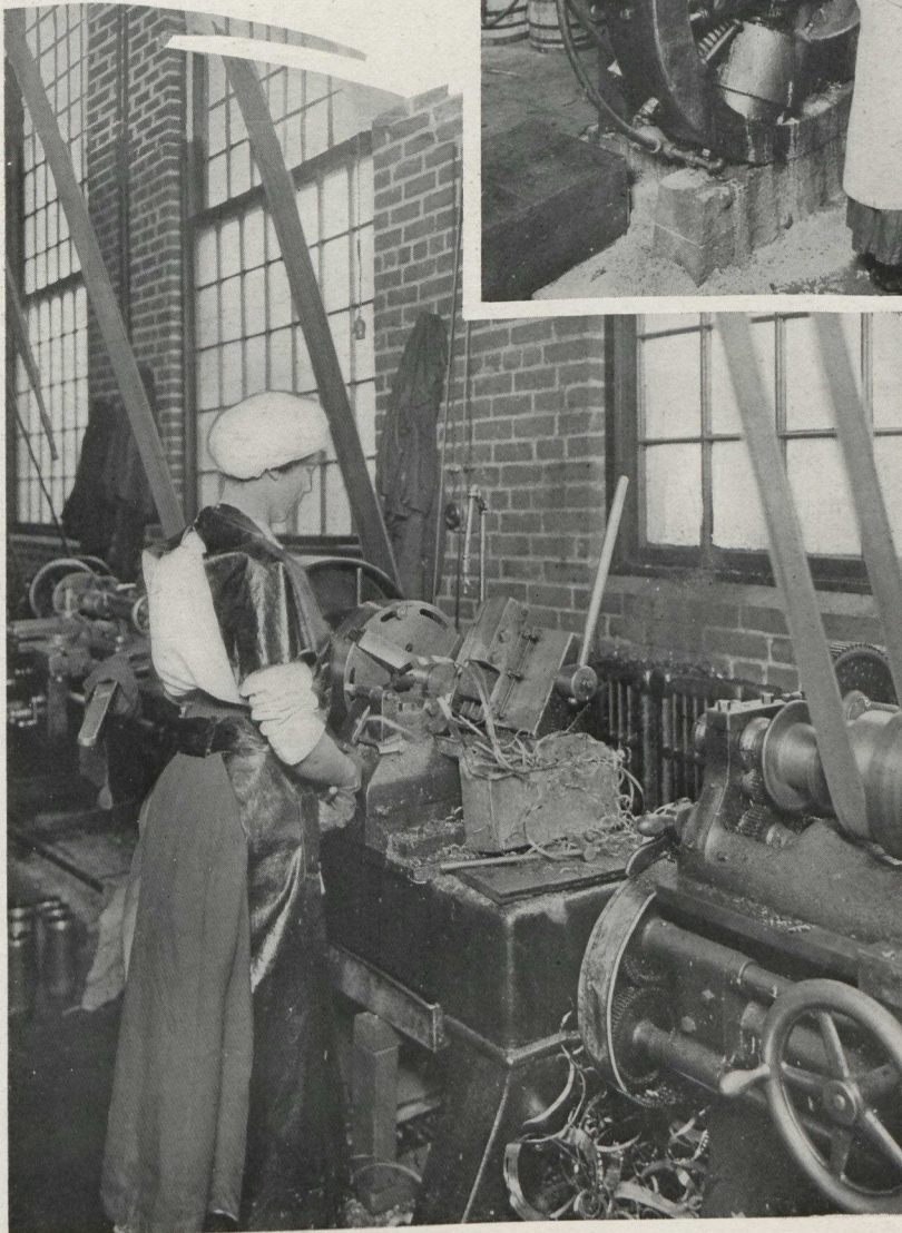
Turning Copper Driving Band, 18-pounder Shrapnel
