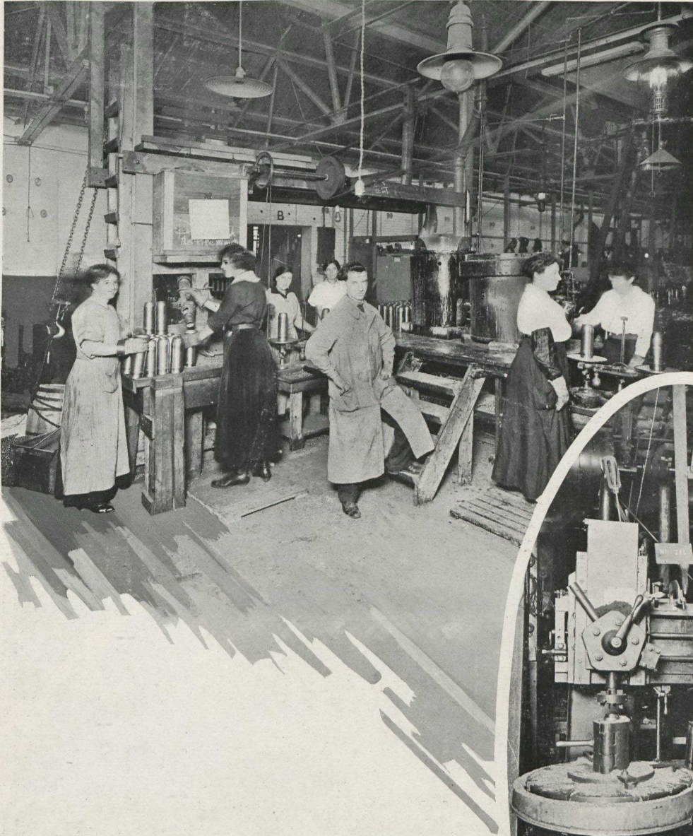
Screwing in and Rough Turning the Brass Socket.
