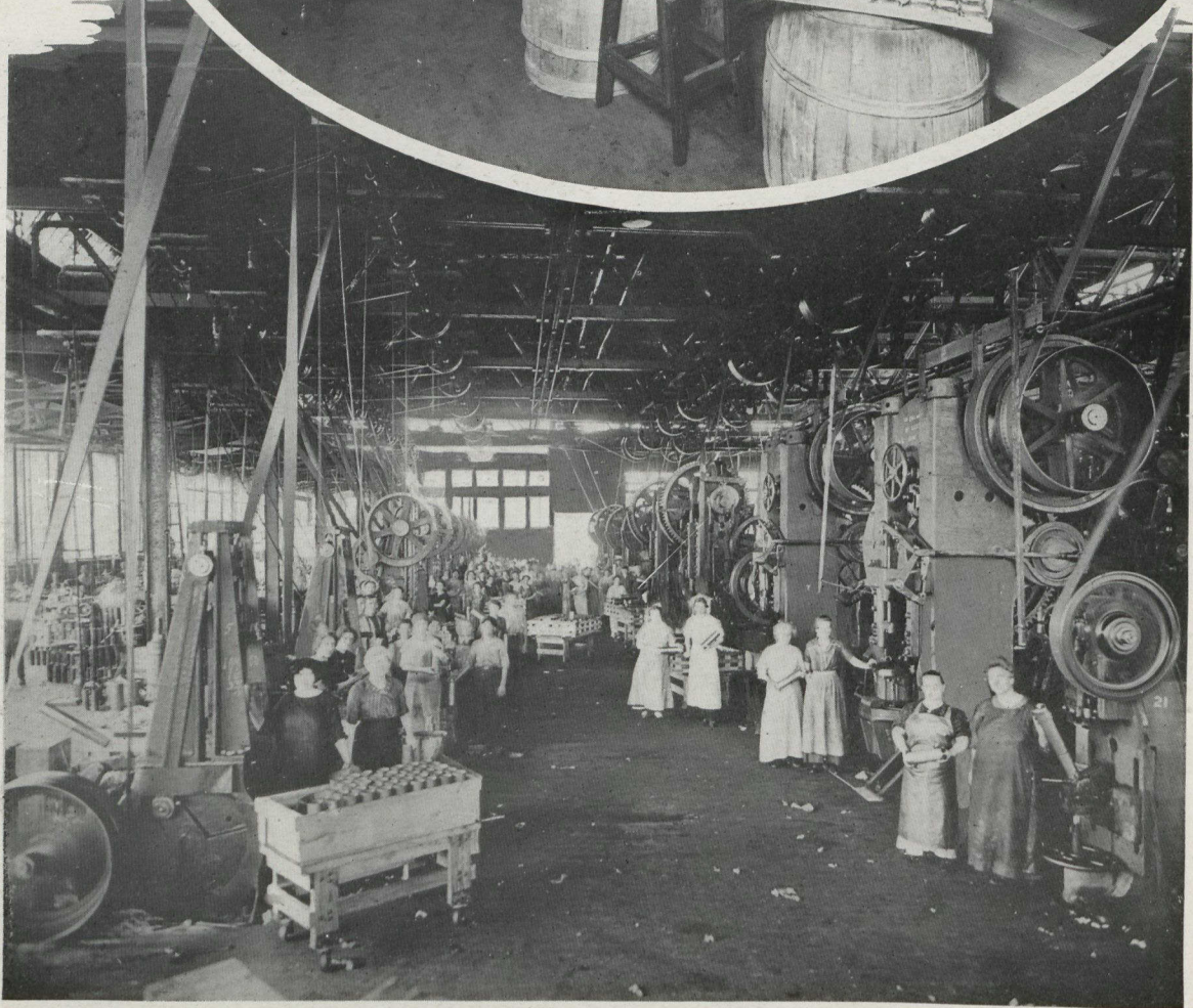
General View of Shop and Bank of Power Presses on Cartridge Cases for 18 Pounds.
