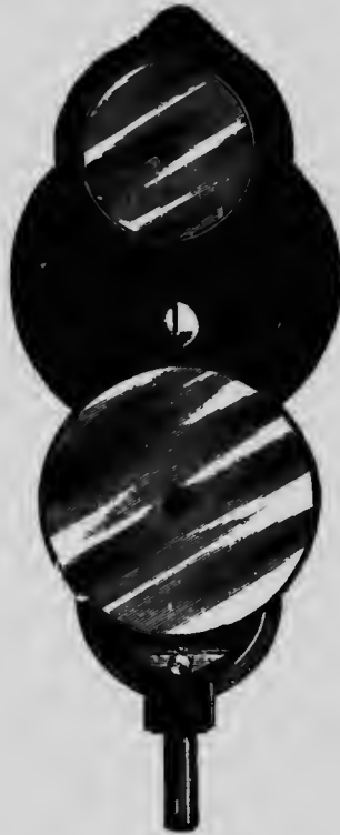
Fig. 586.—The ophthalmoscope. The small upper mirror is for direct, the larger for indirect illumination.
