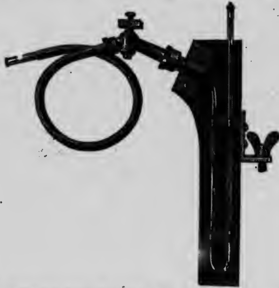
Fig. 273.—The Manometer of Ludwig's Kymograph. It is also shown in fig. 276, D, C, E. The mercury which partially fills the tube supports a float in the form of a piston, nearly filling the tube; a wire is fixed to the float, and the writing style or pen fixed to the wire is guided by passing through the brass cap of the tube; the pressure is communicated to the mercury by means of a flexible metal tube filled with fluid.
