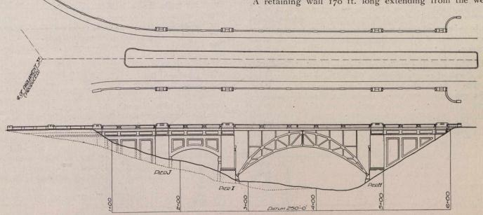
Fig. 1.-Plan and Elevation of the Proposed Rosedale Section of the Bloor Street Viaduct, Toronto.
