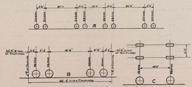
Fig. 3.-Loading Diagrams for Cars and Motor Trucks.
