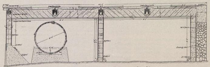
Fig. 4.—Cross-section of Park Terrace and Pipe Line.
