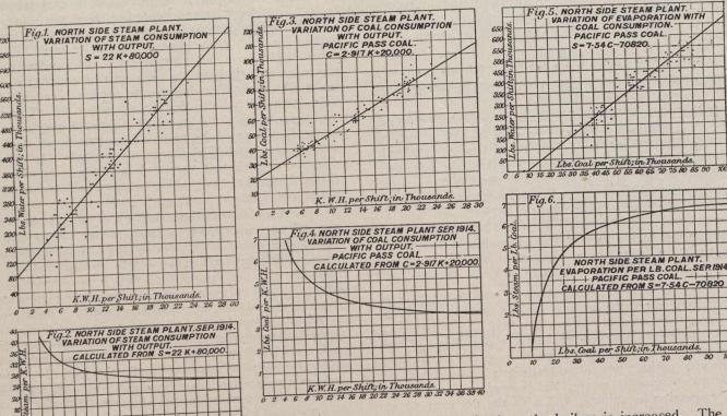
deduced that at an output of 80,000 kw.-hours per shift, which is the rated capacity of the station, the steam consumption would be 23 lbs. per kilowatt-hour. The consumption evidently tends to a limiting value of 22 lbs. per kilowatt-hour with an infinite load on the station.
