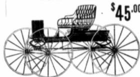
Study the construction of the wagon carefully; every part is made of first-class material and finished equally as good as the highest-priced vehicles. Wheels—1-in. rims, 40-in. front, 44-in. rear, Sarvin patent. Seat—Morrocofine trimmings, swell side stick seat, spring cushion. Gear—Double reach, rear king bolt, fifth wheel, 15-16 long-distance axle. Body—24-in. wide with patent leather dash. Color—Deep black with green gear.
