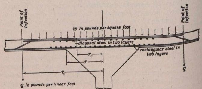
Fig. 2.—Section of Flat Slab.
