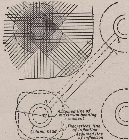
Fig. 1.—Plan of Flat Slab.
