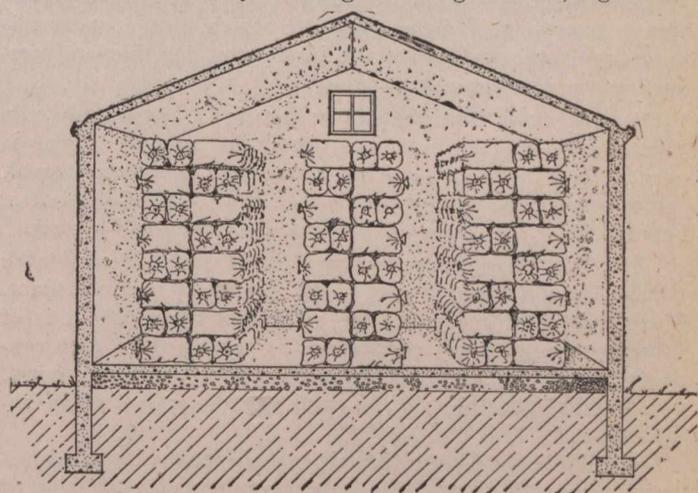
**Cross-Section of Concrete Storage House with Cement Correctly Piled.**
