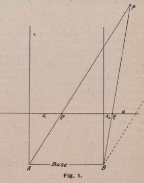
Consider a single photograph and let lines be drawn on it representing the horizon and principal line of the picture. This will divide the photograph into quadrants and the coordinates x and y of any point therein may be measured by means of a comparator. The actual values of these quantities cannot, however, be determined until their distances from the station are measured and this distance may be obtained from a stereoscopic pair.
