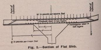
The value of this ratio is taken as 0.1, which has been shown by experiment shown by experiments to be a fair value for concrete of 1:2:4 proportions.
