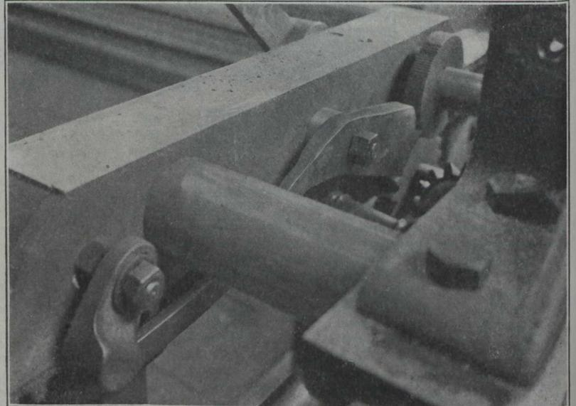
Clamping Mechanism of Cattle Guard Machine.
