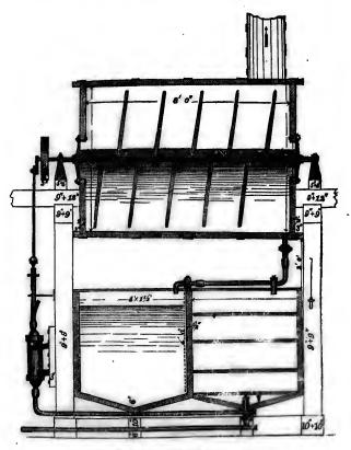
Horizontal Washer and Tanks,-Longitudinal Section.
