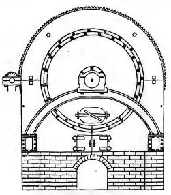
Revolving Retort.-Front Elevation.
