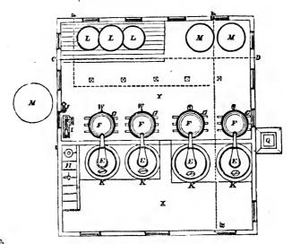
Coal Oil Refinery Plan .- 600 gais. Capacity per Diem,
