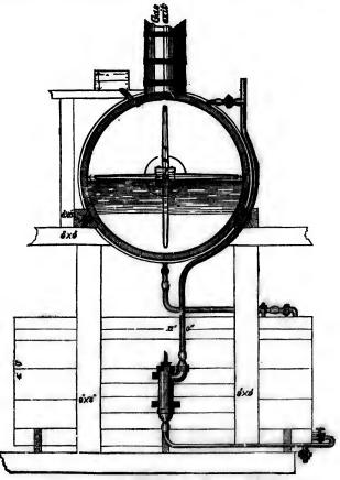
Horizontal Washer and Tanks .-- End Elevation and Section.
