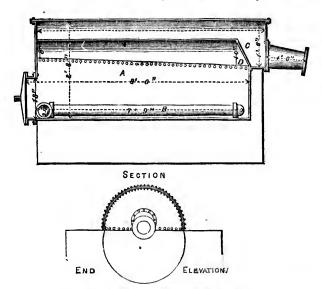
Retort for Bituminous Clays, Asphaltum, etc.
