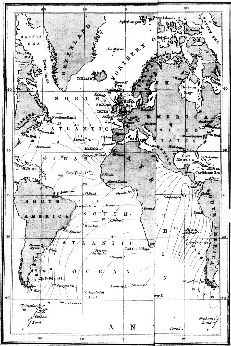
The pecked lines show the progress of the Tide Wave hour by hour. — The figures must not be understood as showing the local time of High Water.
