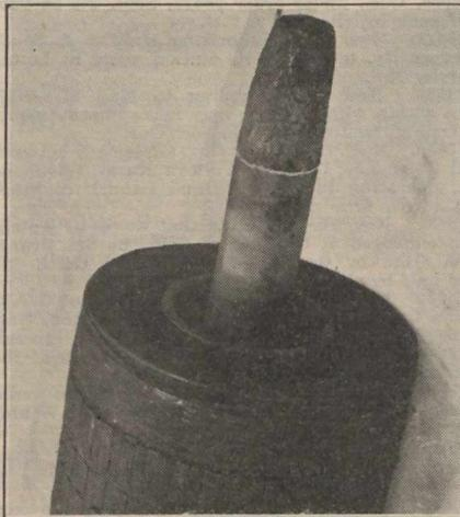
Fig. 2. Repairs to Armature Shaft.
