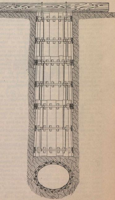
FIG. 3. Shaft lined with corrugated iron. Scale 1/34.
