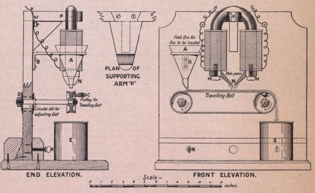
wound with 18 B.W.G. copper wire. Two special pole pieces (N) are provided; they are slotted to allow of the adjustment of the air gap.
