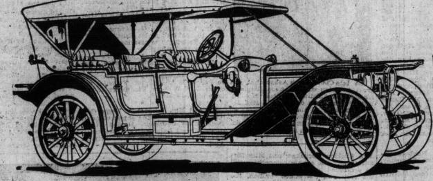
The "American Traveler" (Type 56), \$6000. Six passengers. Wheel base 140 inches; tires 41x4% front and rear on demountable rims. Regular equipment includes: top and top boot; five lamps, side and tail lamps electric, supplied by battery separate from ignition battery; Prest-O-Lite tank; Bosch magneto and storage battery; two extra rims; shock absorbers; foot rest; robe-rail; tire holders; horn; jack; tools and tire repair outfit. Weight with standard equipment 3850 lbs. Our Claims
