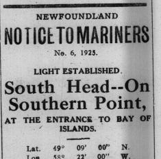
Lon. 58° 22' 00" POSITION-On South Head, at the entrance to Bay of Islands, CHA RACTER - A double Flashing WHITE ACETYLENE GAS Light, giv ing 15 flashes per minute.
