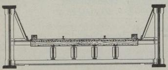
Fig. 3.-Through Plate Girder.
