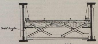
Fig. 2.—Half Deck Plate Girder.
