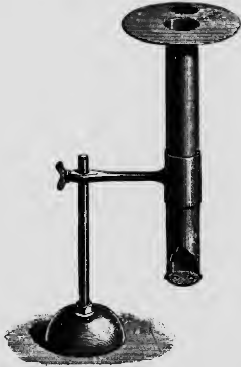
FIG. 12.—CAMERA TUBE FOR USE WITH OLIVER'S HÆMOMETER.
