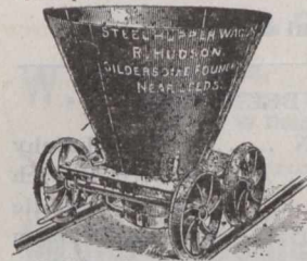
27—Hopper Wagon, with Slide Door
