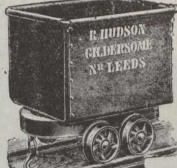
70—R.H.'s Patent Steel Mining Wagon
