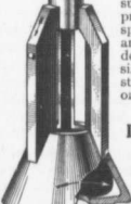
Dist-arrester chamber with part of side broken away to show how the impurities are collected.
