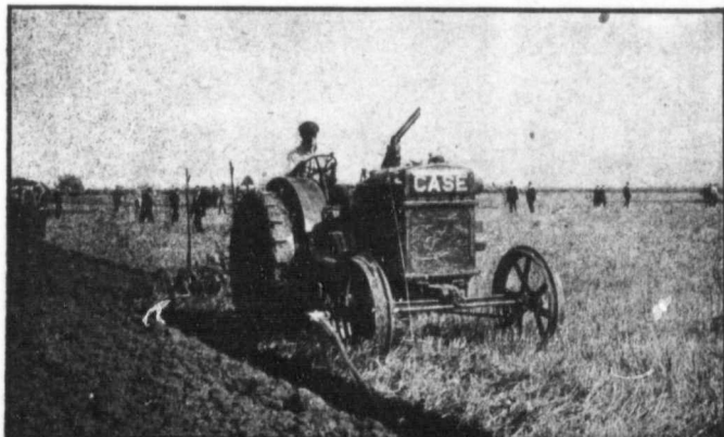
The Outfit that took Second Prize. A Grand Detour 3 Bottom Rigid Beam Plow and a Case 15-27 Kerosene Tractor
