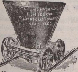
27—Hopper Wagon, with Slide Door
