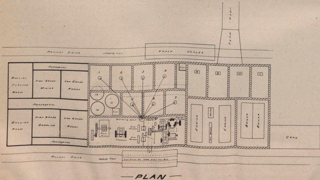
NOTE: Bins No 1 to 7 are for Low Grade Ore (Reject) Directly under these are Stone Rooms for High Grade Ore in bags. Hoppers No 12, 13, 14 are for High Grade Rejects which are to be bagged. Bins 8, 9, 10, 11 are for Low Ore loaded from No 1.
