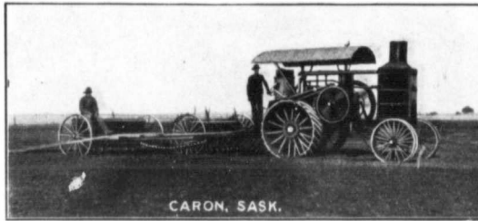
A Hart Parr 22 h.p. Gas Tractor pulling two drills. Outfit of A. H. Powell, Caron, Sask.
