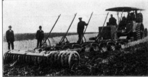
A Robt Bell Steam Tractor pulling a 10 bottom 14 inch John Deere Engine Gang and a Fulton subsurface packer at Gainsboro Sask. Outfit of Ed. Bourke.
