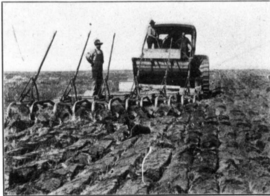
Phillips and Heathers Avery undersmounted Engine pulling a 12 bottom 14 inch John Deere Engine Gang at Magrath, Alta.
