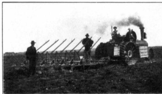
A Case 25 H.P. Steam Tractor pulling a 7 bottom 14 inch Cockshutt Engine Gang, Outfit F. F. W. Hunter, Stonewall, Man.
