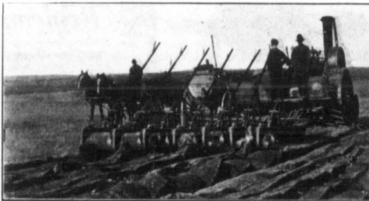
A Sawyer-Massey Steam Tractor pulling a 7 bottom 14 inch Cockshutt Engine Gang, Outfit E. Evenson, Moose Jaw
