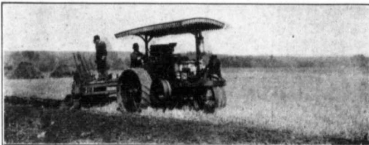
A Russell Gas Tractor pulling a Sioux Falls Engine Gang.
